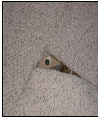
**Quarter-sized port to collect sub-slab air**
