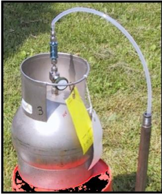
**Summa Canister to collect indoor and sub-slab air**
